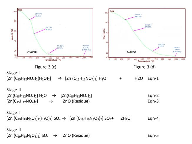
From the thermo gravimetric analyses of AVOP Zn complex shown in figure-3 (c), it was observed that the compound is thermally stable up to 184°C. The zinc complex decomposes with the formation residue with percentage of 9.817% which is close to the theoretical value of 8.969%. The decomposition of the ZnAVOP complex occurs according to the equation 6.
