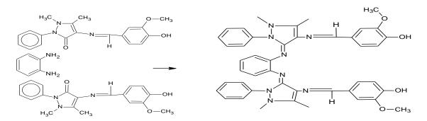
Scheme 1.3 Preparation of ligand AVOP (4-aminoantipyrine vanillin o-phenylenediamine Schiff base)
